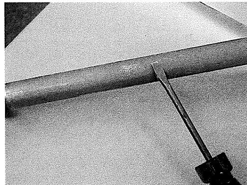
Galvanized Iron- Dull steel color. Magnet will stick to it.
